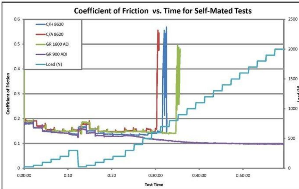
**Figure 11: A comparison of carburized and hardened and Carbo-Austempered™ steels to Grades 900 and 1600 ADI in a step load galling test. The ADI 900 (purple line) did not gall in this test.**
