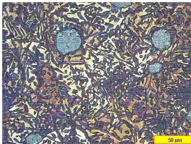
**Figure 5: This microstructure of an ADI Grade 750 illustrates the mixed proeutectoid ferrite (light tan) and ausferrite (light brown to purple) microstructure.**
