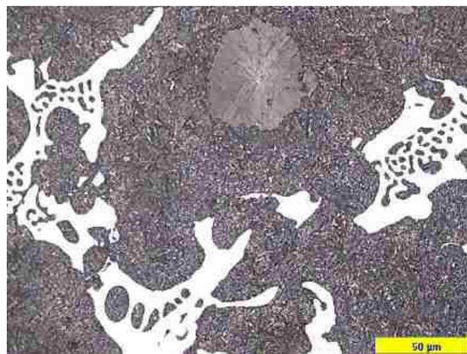
**Figure 2:** A photomicrograph of a Carbide ADI microstructure showing as-cast alloy carbides, a graphite nodule and a matrix of Ausferrite is shown. (From Hayrynen et al<sup>5</sup>).
