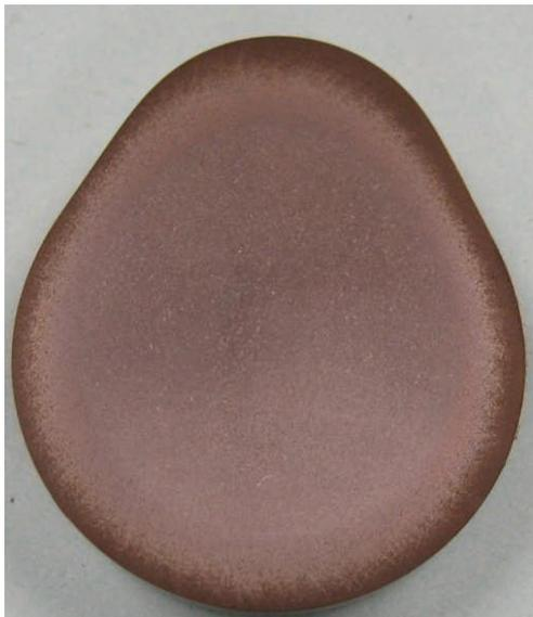
**Figure 1:** This is a cross-section view of an LADI™ cam lobe that has been etched with 5% Nital to show the controlled-depth Ausferritic case on a largely ferritic core. (From Bixler et al<sup>4</sup>)
