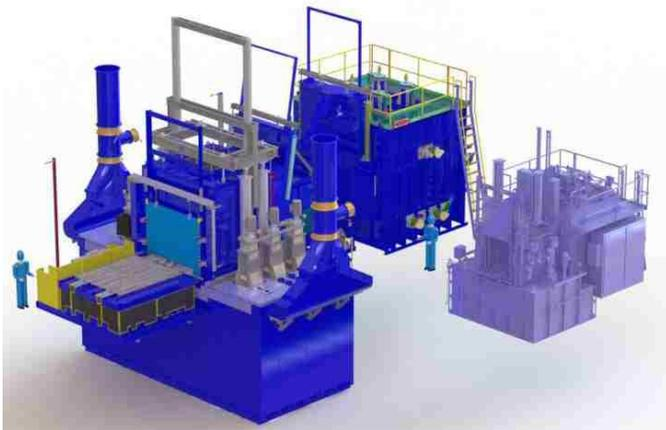
**Figure 3: The AP Monster Parts™ Division's 7m<sup>3</sup> AFC-Holcroft UBQA furnace is shown side by side with a 0.8 m<sup>3</sup> UBQ furnace for comparative effect.**
