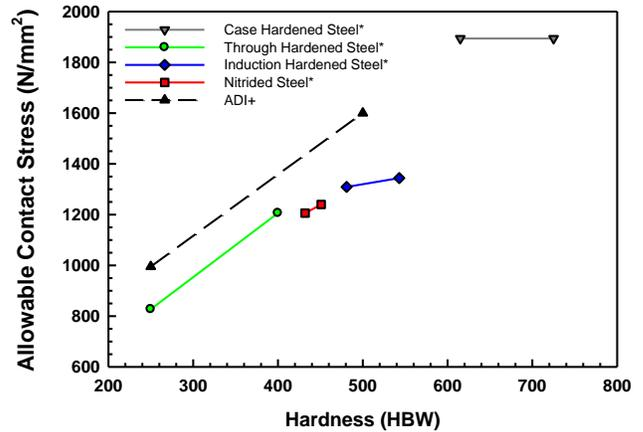
**Figure 6: A comparison of the allowable contact stress vs. hardness for ADI and various steel-based material/process combinations.**
