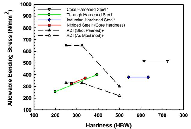
**Figure 7: A comparison of the allowable Gear Tooth Root Bending Fatigue vs. hardness for ADI and various steel-based material/process combinations.**
