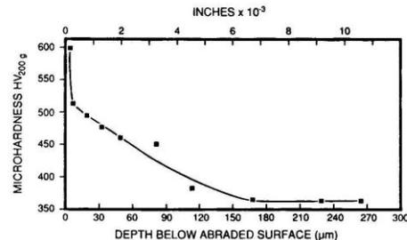
**Figure 9: The depth of the transformed layer in ADI after exposure to a high normal force is illustrated by an increase in microVickers hardness near the surface. From the Ductile Iron Data Book for Design Engineers<sup>13</sup> – [www.ductile.org](http://www.ductile.org).**
