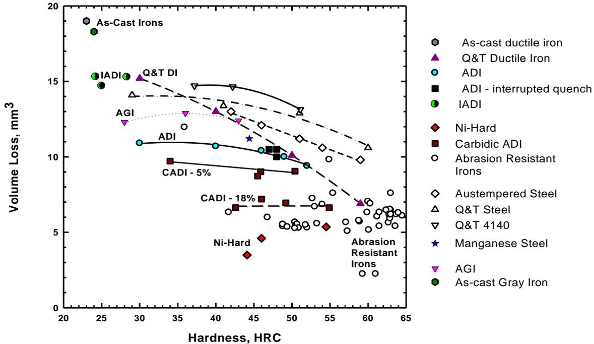
Figure 10: A comparison of the pin abrasion test results for ADI, IADI and CADI™ compared to competitive materials as a function of matrix hardness. Testing was completed in accordance with ASTM G132-96(2007).
