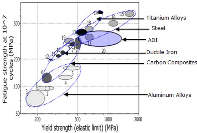
**Figure 8: This figure compares allowable rotating bending fatigue vs. yield strength for various groups of materials. (Illustration derived from Keough et al<sup>9</sup>.)**
