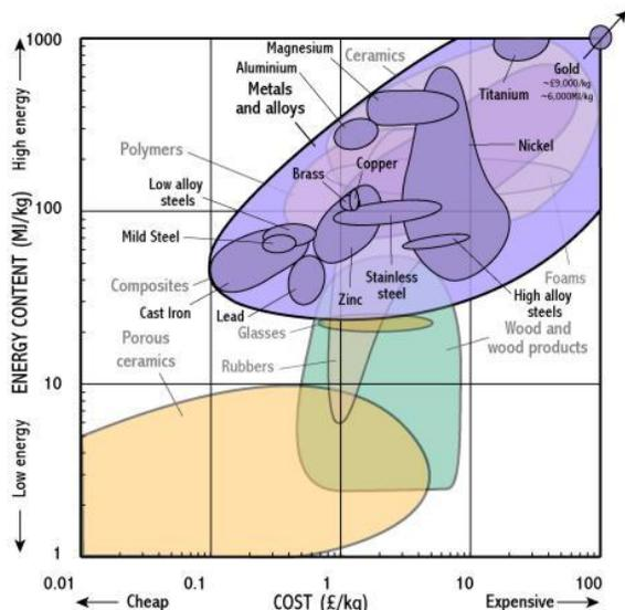
**Figure 4: Energy content (embodied energy) is plotted versus cost (£UK) for various metallic materials from Cambridge University in this figure, [www.msm.cam.ac.uk](http://www.msm.cam.ac.uk).**
