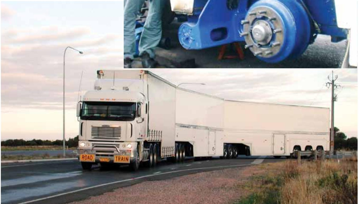
Fig. 2. Pictured is the cast ADI bracket installed on the truck trailer as well as the truck and trailer in action.
