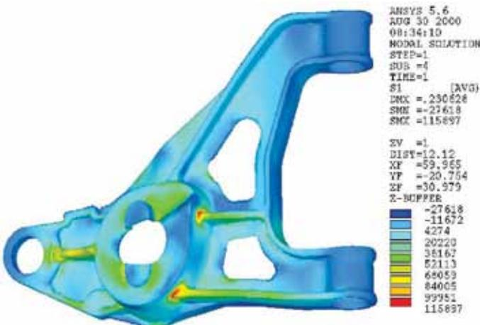
Fig. 4. Shown is the analysis using the 4G load on the cast design that helped identify the hot spots.
