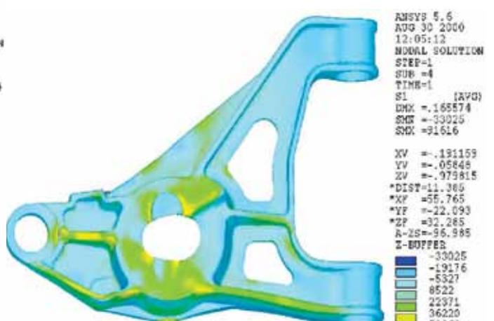
Fig. 5. Pictured is the final cast ADI control arm design during structural analysis.
