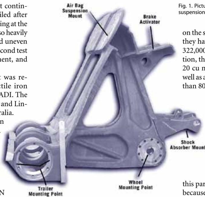
Fig. 1. Pictured is the cast ADI independent track trailer suspension bracket.
