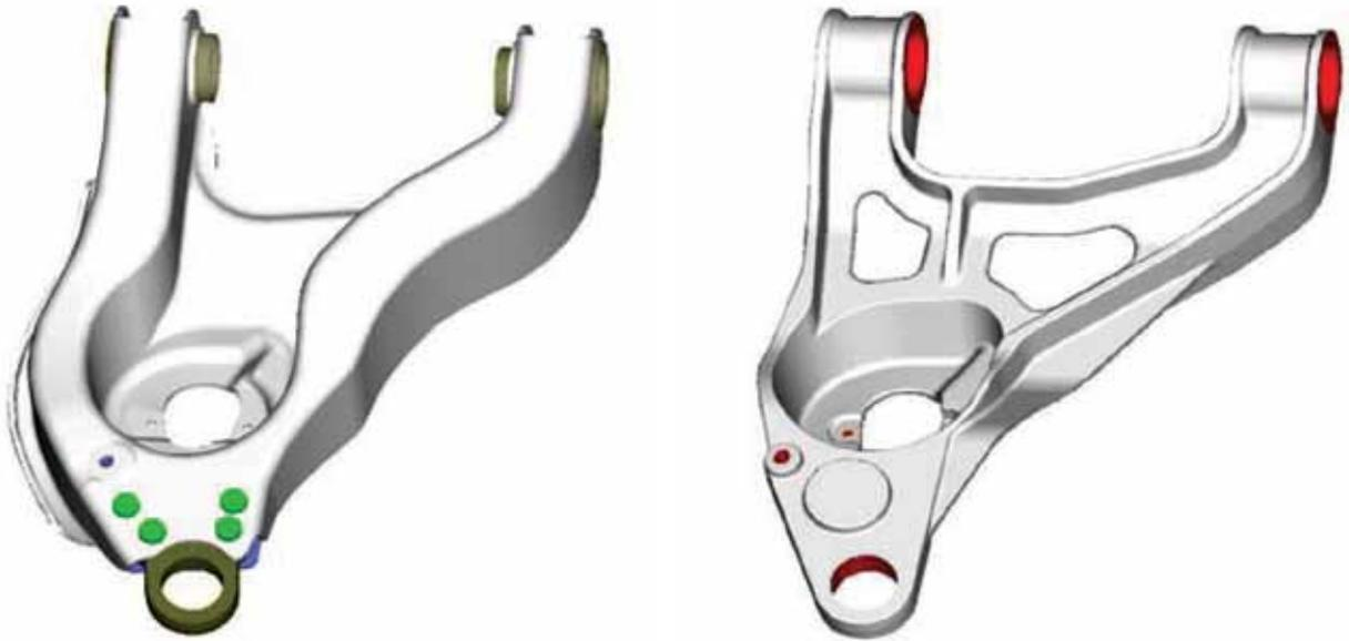
Fig. 3. Pictured is the stamped steel control arm design (l) and the initial cast ADI design (r).
