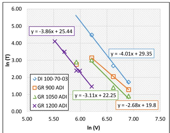
**Figure 3:** The effect of cutting speed on tool life in ADI and 100-70-03 DI (T = tool life - min; V = cutting speed – ft/min).
