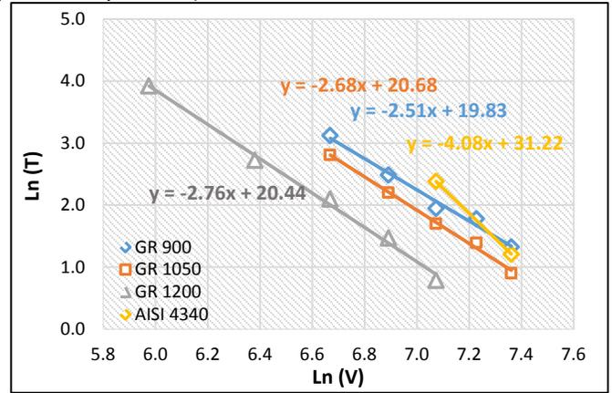
**Figure 3:** The effect of cutting speed on tool life in ADI and AISI 4340 (T = tool life - min; V = cutting speed - ft/min).
