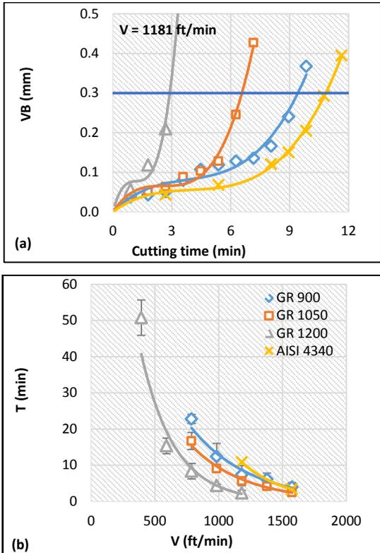
**Figure 2:** (a) Tool wear behavior during machining of ADI and AISI 4340 at cutting speed of 1181 ft/min; (b) The effect of cutting speed on tool life in different ADI grades and AISI 4340.
