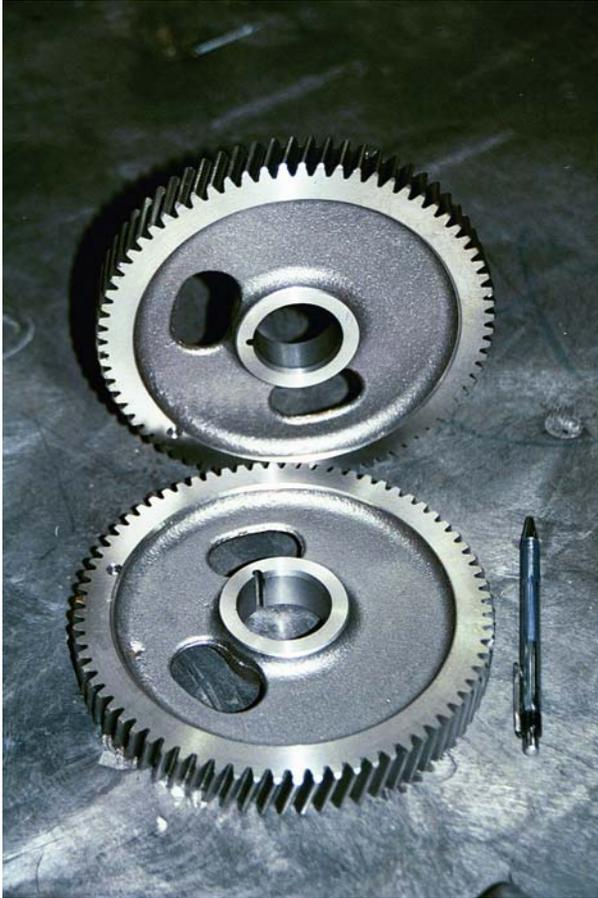
**Figure 11: Diesel engine timing gears made of ASTM A897-03 Grade 230-185-01 ADI (approximately 480 HBW) [12]**
