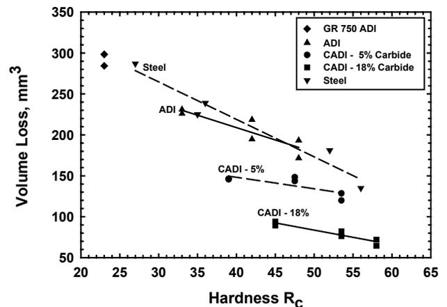
**Figure 6: Dry Sand/Rubber Wheel Abrasion results for various austempered ductile irons and steel.**
