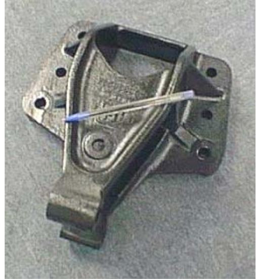
**Figure 10:** A heavy truck suspension bracket made of ASTM-A897-03 Grade 130-90-09 ADI (~300 HBW). [12]
