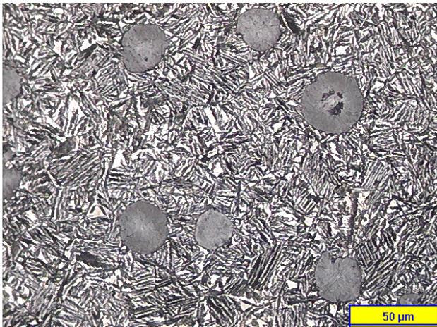
**Figure 1: Photomicrograph of Austempered Ductile Iron. The ausferrite matrix typically consists of acicular ferrite (needles) and high carbon austenite (light colored phase).**
