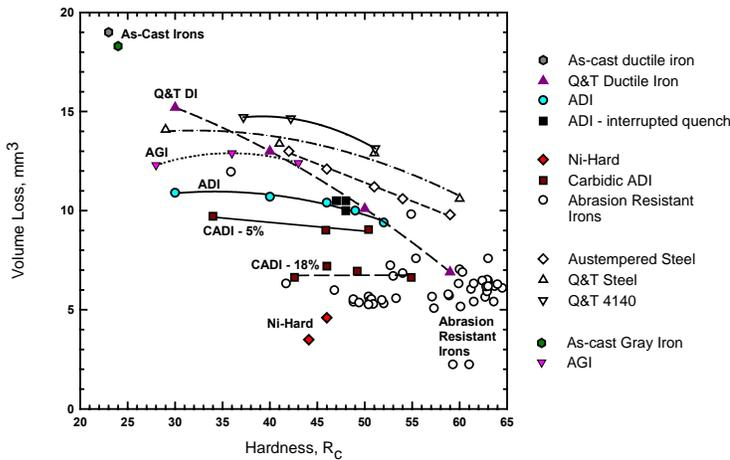
**Figure: 4 Pin Abrasion Data for various cast irons, austempered ductile irons, steel and abrasion resistant irons. Abrasion resistant iron data from the Abrasion-Resistant Cast Iron Handbook. [7]**
