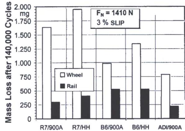
**Figure 3: Mass loss after 140,000 cycles for various wheel/rail material combinations. This figure shows that both the ADI wheel and the steel track wore less than the steel/steel pairings in a test with a 1410N normal force and 3% slip. (From Mädler)**
