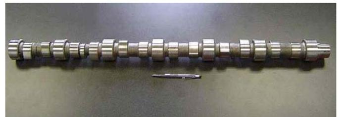
**Figure 8:** Typical ductile iron automotive camshaft.
