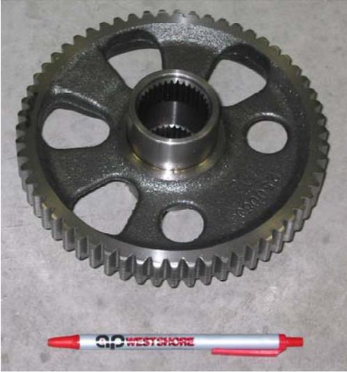
**Figure 9.** This is the final drive gear for an off-highway utility vehicle. It is austempered to grade ASTM A897-03 175-125-04 after machining. [12]
