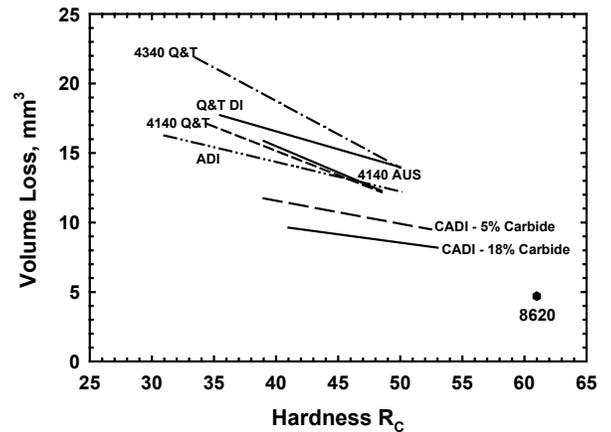
**Figure 5: Wet Sand/Rubber Wheel Abrasion results for various ductile iron, austempered ductile irons and steel.**
