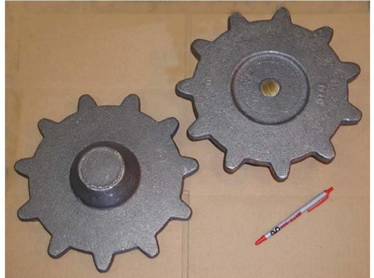
**Figure 12: The sprocket shown in this figure replaced an induction hardened sprocket. The ASTM A897-03 Grade 150-110-07 sprocket teeth wear comparably to their induction hardened counterparts but they are much tougher and not subject to breakage. [12]**
