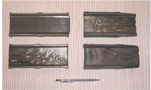
**Figure 7.** In a side-by-side test of shotblast vanes, high-Cr white iron (top left) out performed CADI (bottom left). In a similar test on a different machine, high-Cr white iron (top right) outwore an ASTM A897-03 Grade 230-185-01 ADI (bottom right). Notice the wear pattern of the ADI in the absence of carbides.
