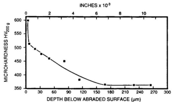
**Figure 2: Microhardness as a function of depth for an abraded surface of ADI. (From Ductile Iron Data for Design Engineers.[1])**
