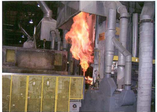
Parts being loaded into an austempering furnace.
