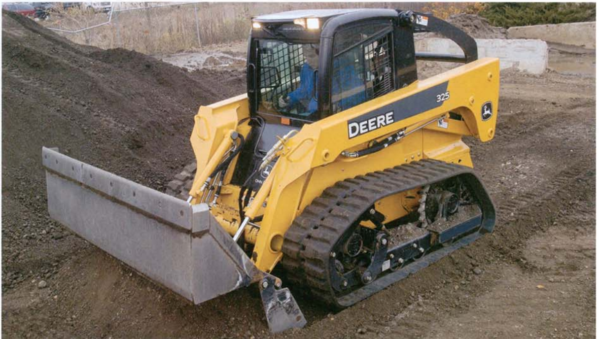
The Loegering VTS track system can be installed on a number of different skid steers.
