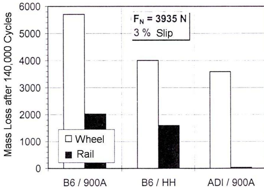
Figure 4- Mass loss for various wheel/rail material combinations at 3% slip and  $F_N = 3935\text{ N}$
