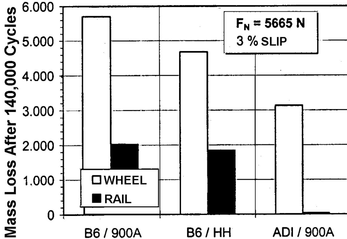
Figure 5- Mass loss for various wheel/rail material combinations at 3% slip and  $F_N = 5665\text{ N}$
