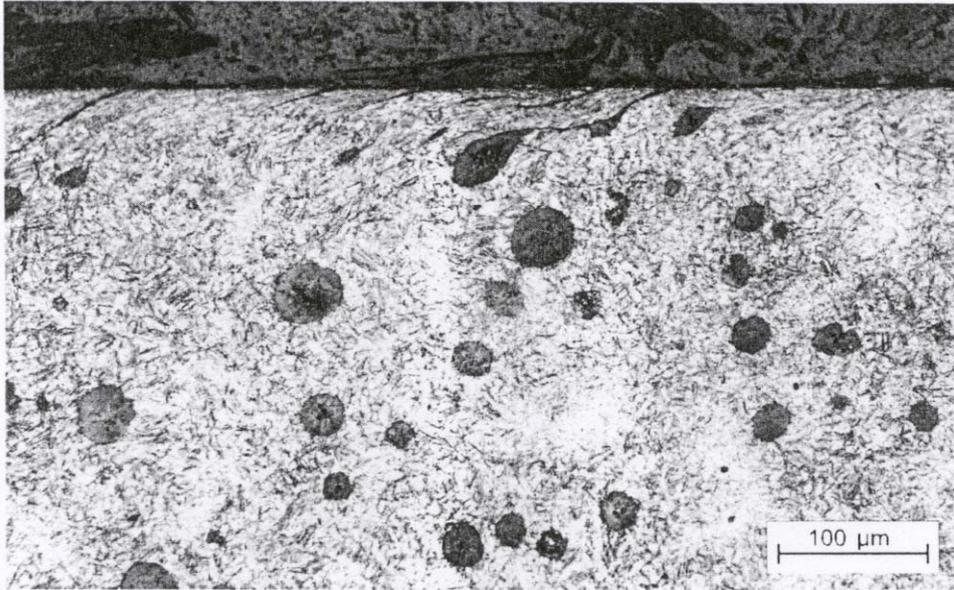
**Figure 6- Surface microstructure of the ADI test sample after roll/slip testing at  $F_N=5665$  N**
