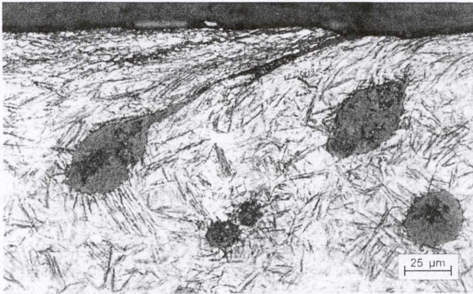
**Figure 7- Surface microstructure of the ADI test sample after roll / slip testing at  $F_N=3935$  N**
