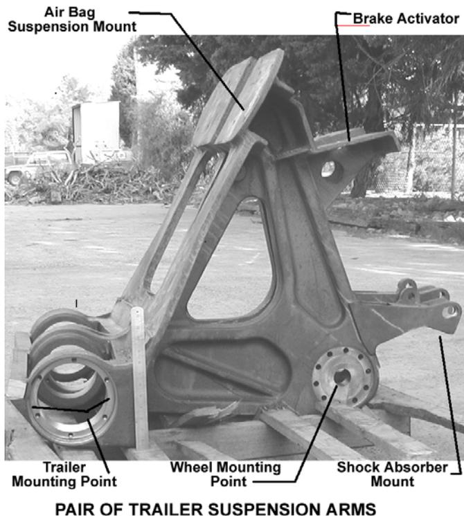
**Figure 6: ADI Independent Truck Trailer Suspension Brackets.**
