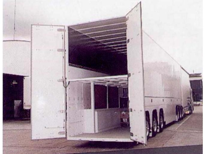
**Figure 4: Interior View of a Trailer Utilizing the Independent Suspension and a Double Deck Arrangement.**
