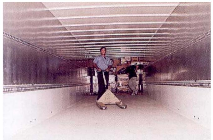
**Figure 5: The Double Levels on the Interior of the Truck Allows Full Walk-Through Capability**
