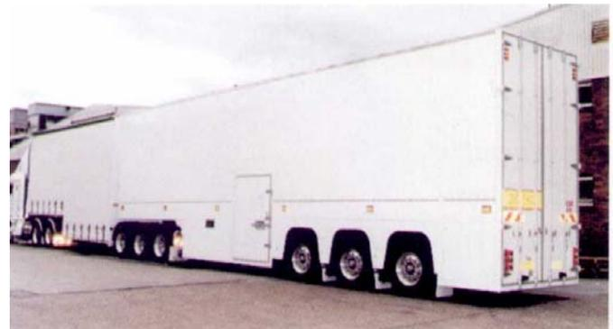
**Figure 1: Linehaul truck trailer with new independent suspension system.**
