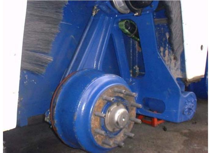
**Figure 7: Independent Suspension Bracket as installed**
