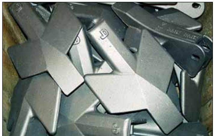
Fig. 9. These John Deere LaserRip ripper points were produced in CADI for wear resistance and toughness in abrasive, rocky soil.
