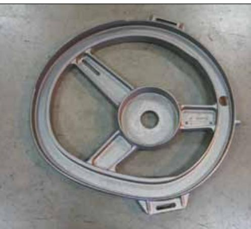
Fig. 3. This large austempered gray iron cam wheel is used in a harvesting machine.
